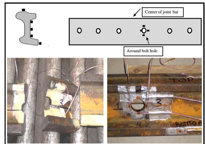
Figure 2. Strain gage and saw cut locations
