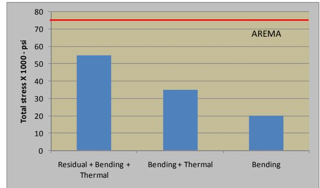
Figure1. Effects of residual stresses on total stresses
